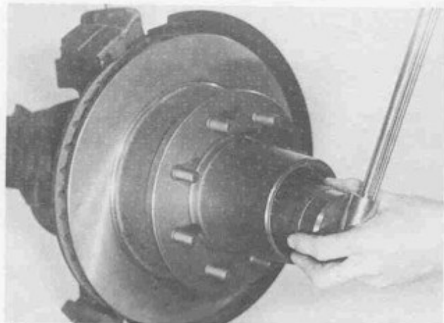
Figure 53 1019-53 To adjust wheel bearings, torque inner adjusting nut to 50 Lb. Ft. (68 N·m) to seat bearings. Rotate hub, then back off inner adjusting nut one-fourth turn maximum. Assemble lock washer, turn nut to nearest hole in washer. Assemble outer locknut and torque to 50 Lb. Ft. (68 N·m). Final bearings adjustment to be .001-.010 (.03-.25 mm) total end play.
