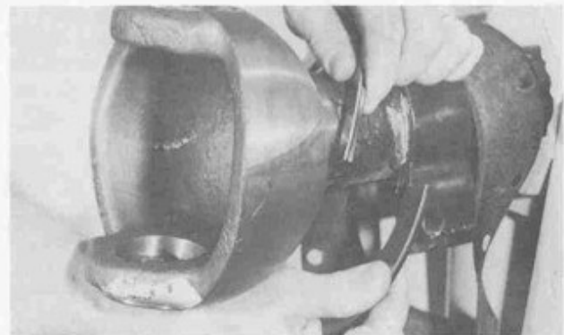
Figure 33 1019-33 Assemble new oil seal with the metal part of the seal towards the end of the axle. Spread split of seal just enough to slip over the tube of the axle.
