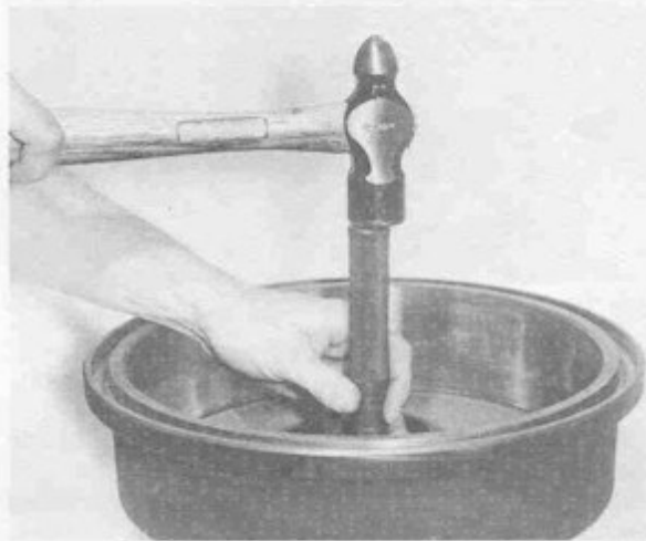
Figure 12 1019-12 Remove inner and outer wheel bearing cups. Tools: #D-255 Cup Remover, #C-4171 Handle.
