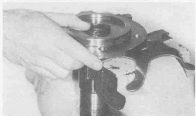
Figure 69 1019-69 Assemble grease seal into spindle. The lip of the seal is to be directed away from the spindle.
